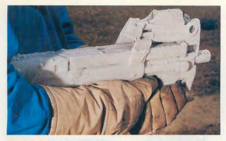
FN has subjected the P90 to the usual dynamic environmental tests with great success. More than 250,000 rounds were fired during its development. Photo: courtesy FN Herstal
